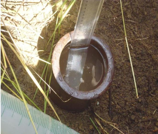
Figura 7: Infiltrômetro de Hills.
